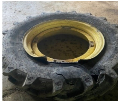
A Wheel And Tire Damaged By A Broken Boom
